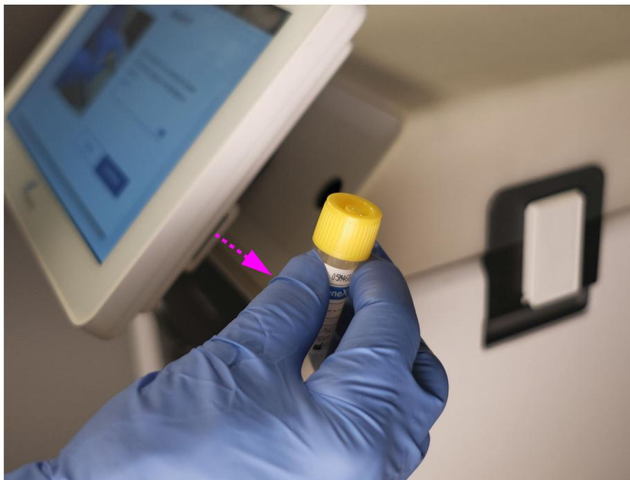
**Figure 3-13. Correct Placement for Scanning a Sample**
