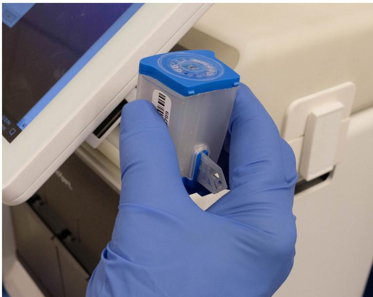
**Figure 3-20. Correct Placement for Scanning a Cartridge**
