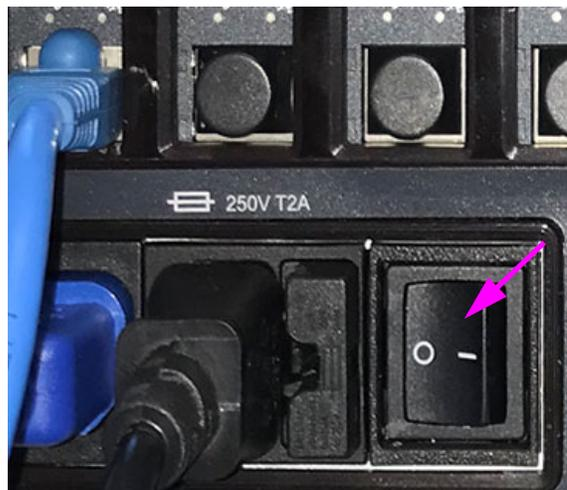
**Figure 3-48. GeneXpert Xpress Hub Power Switch (Rear of Hub)**
