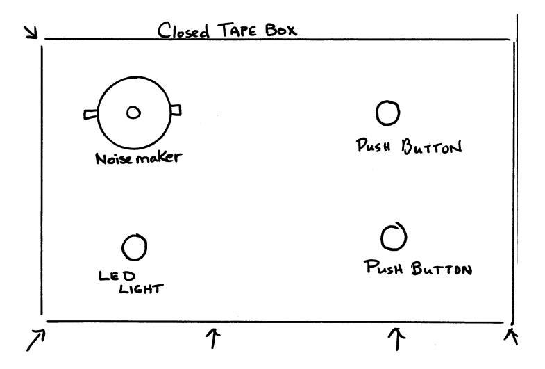
Seal the tape box with black electrical tape so residents cannot open the case or expose the wiring.
