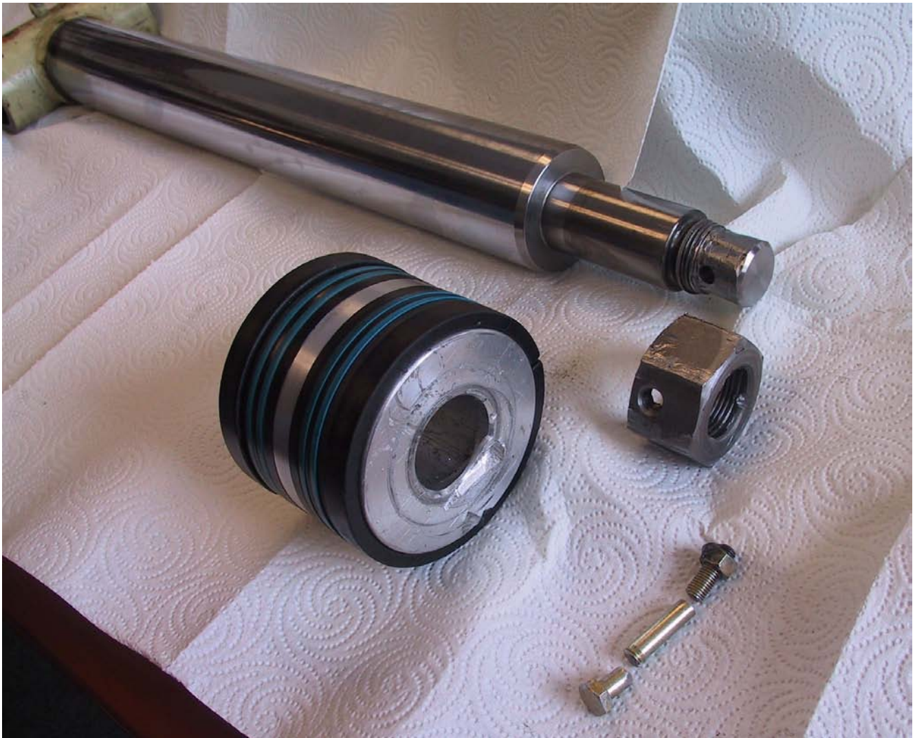
Photo 6. A bolt had been inserted through the hex nut and the rod and it was fastened with a nut. The bolt broke into three pieces during the incident and caused the cylinder to fail.
