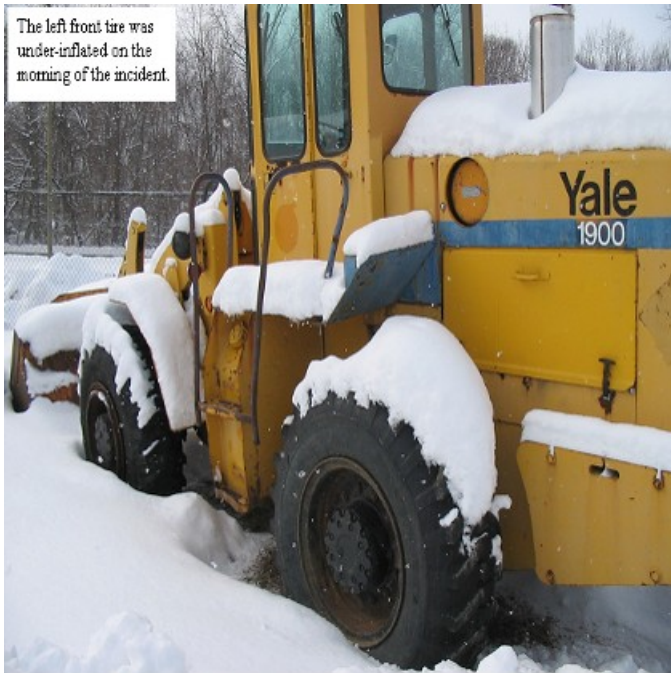
Photo 2. The loader that was operated by the victim on the morning of the incident. The left front tire was under-inflated at the time of the incident. (Photo courtesy of OSHA)
