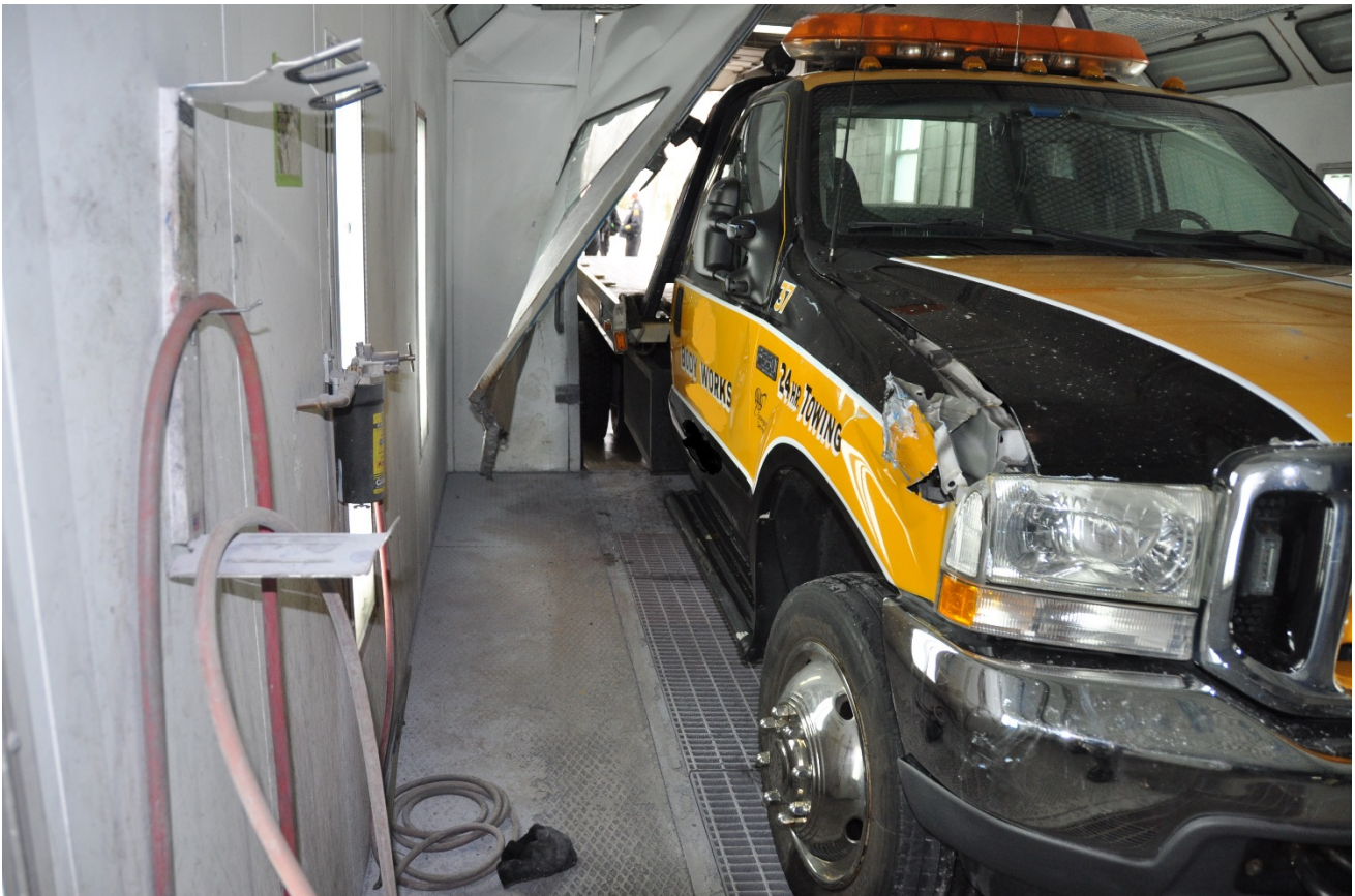
Photo 2. The victim was crushed and pinned between the paint booth door and the passenger side of the truck (photo courtesy of OSHA).
