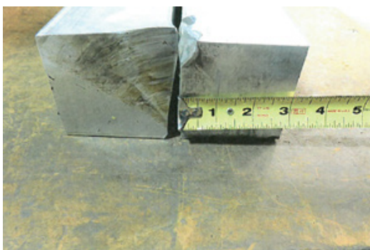
Photo 4: In-house fabricated aluminum safety blocks with deformed corners and scraped metal face. (Photo courtesy of OSHA)
