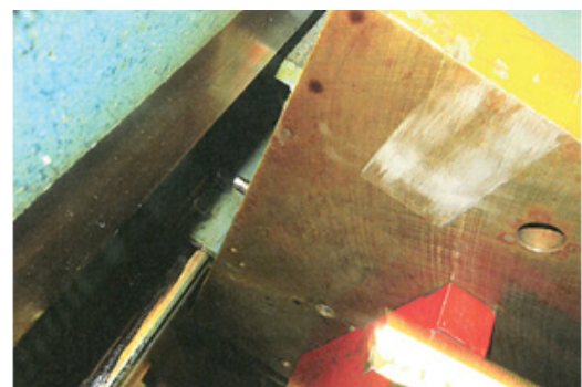
Photo 5: Picture of mechanical press ram indicating where safety block had been placed. (Photo courtesy of OSHA)
