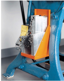
Photo 1: Example of safety blocks with interlock devices. (Photo from EHSToday.com)
