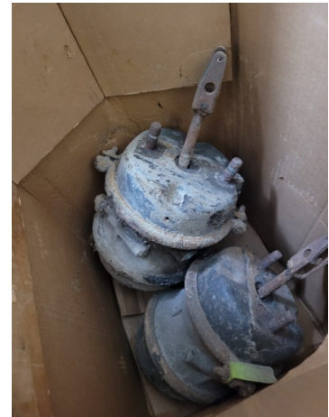
Photo 3: Air brake canisters or 'air cans' involved in routine maintenance of truck braking system
