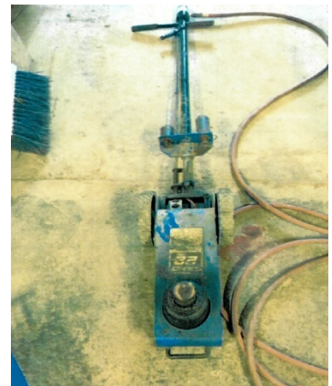
Photo 4: 22-ton pneumatic jack typically used to support truck during air brake maintenance (photo courtesy of PESH)
