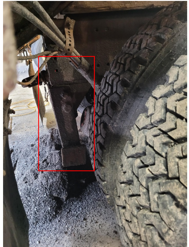
Photo 2: Chipper bar behind right rear tires of truck
