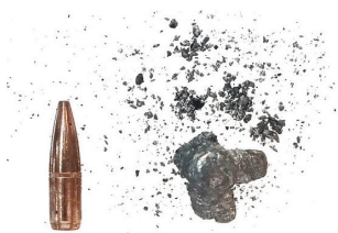
A lead bullet with copper shell before and after firing.
