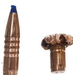
A lead-free copper bullet and shell before and after firing.
